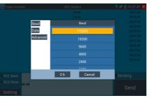
Click "Setting" to choose the baud rate of RS485; it must be the same as the DVR or the Control. keyboard .The DVR or Control keyboard send the code to the tester, if it can be read, the protocol will shown on the upper right, like Pelco D, if not, like P:---
